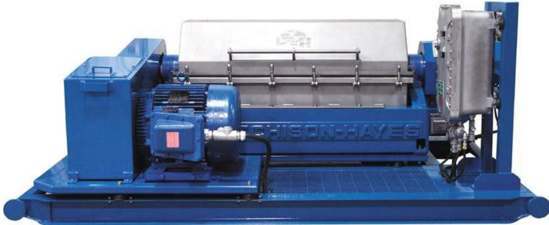
The HH 5500 Standard is a configuration of a drive system for a Decanting centrifuge. This configuration is the most basic of many available configurations. The Centrifuge bowl is driven by a main drive motor and the conveyor is driven through a planetary gear box with a simple torque arm setup.
