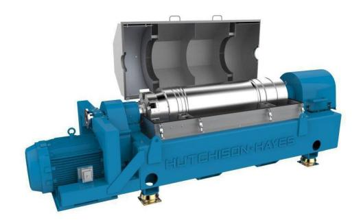
The MegaBowl ™ comes with a standard "VFD Ready" configuration of a drive system for the decanting centrifuge. This configuration allows for a fully variable main and back drive when using a VFD. The Centrifuge bowl is driven by a 150 HP inverter duty main drive motor and the conveyor is driven through a planetary gear box with a 40 HP inverter duty back drive motor.
